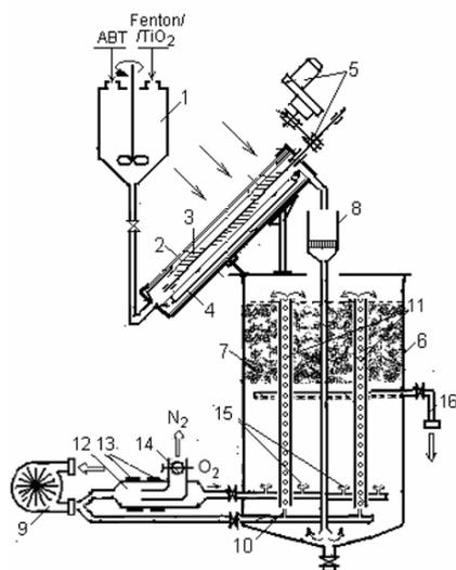
**Fig. 2.1.** The scheme of the combined photocatalytic and biochemical reactors for the destruction treatment of water, containing persistent organic compounds: 1 – inclined framework; 2 – quartz tubes; 3 – brush; 4 – UV-lamps; 5 – motor; 6 – bioreactor’s case; 7 – substrate for microflora fixation; 8 – filter; 9 – air blower; 10 – air inlet; 11 – aerolift; 12 – oxygen enrichment; 13 – magnets; 14 – regulating choker; 15 – bubbling; 16 – outlet for treated water.
