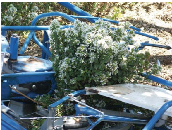
Fig. 18 Mechanization is a necessity for modern essential oil crops growers. In the photo, a prototype of mower modified for harvesting of oregano ( Origanum vulgare L. subsp. hirtum (Link) letswaard). (Photo: A. Carrubba)
