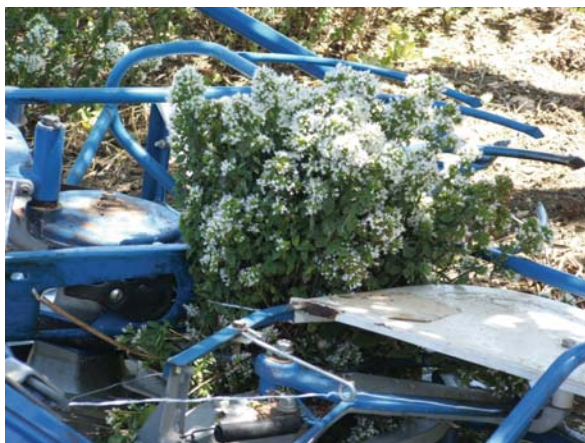
Fig. 18 Mechanization is a necessity for modern essential oil crops growers. In the photo, a prototype of mower modified for harvesting of oregano ( Origanum vulgare L. subsp. hirtum (Link) letswaart). (Photo: A. Carrubba)
