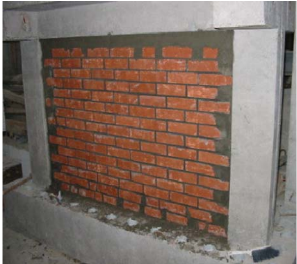
Plate 35 Strengthening of a bare frame by integrated high strength bricks (see also Fig. 19.16 on page 399)
