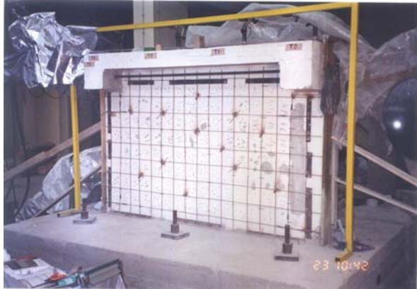
Plate 32 Integrated wall and strengthening by wire mesh (see also Fig. 19.13 on page 398)
