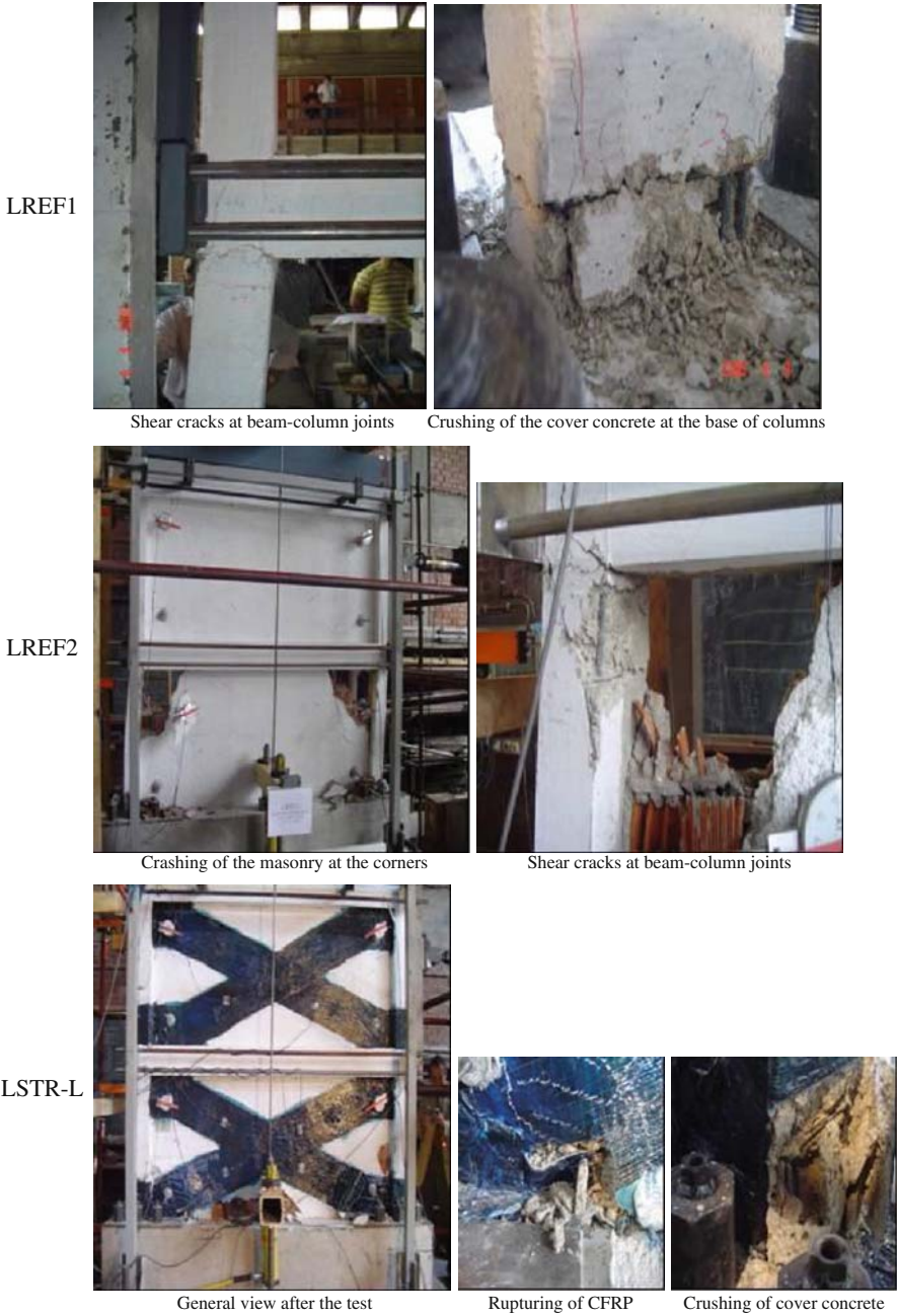
Fig. 18.5 Failure pattern of the test specimens
