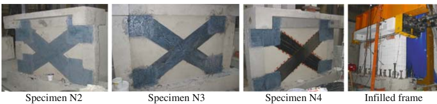
Fig. 19.20 Different CFRP applications and infilled frame specimen (See also Plate 36 in Color Plate Section on page 475)
