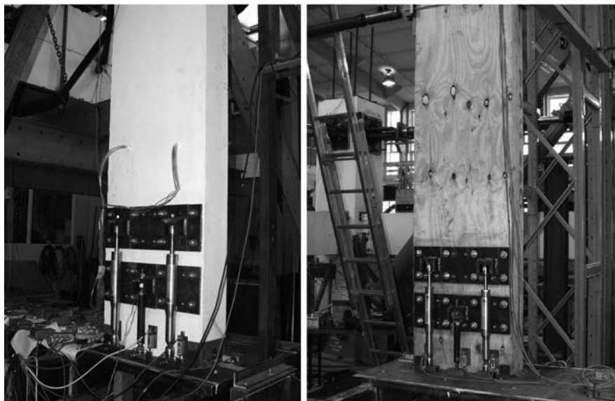
Fig. 13.16 Prototypes of post-tensioned rocking/dissipative concrete and timber walls under shake table tests (after [39])
