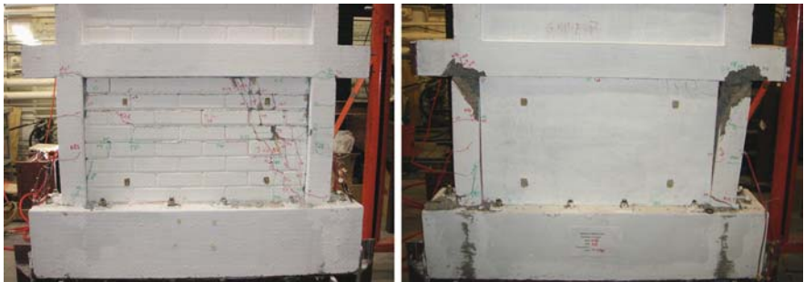
Plate 24 Failure modes of Stanford specimens; (a) reference specimen without retrofit, (b) specimen with ECC layer [10] (see also Fig. 17.7 on page 353)
