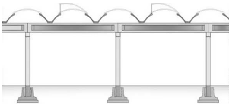
Fig. 10.19 Subtype “3c”: one storey buildings I-beams of and special long span roof elements
