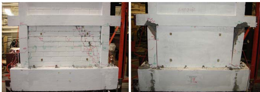
Fig. 17.7 Failure modes of Stanford specimens; (a) reference specimen without retrofit, (b) specimen with ECC layer [10] (See also Plate 24 in Color Plate Section on page 469)
