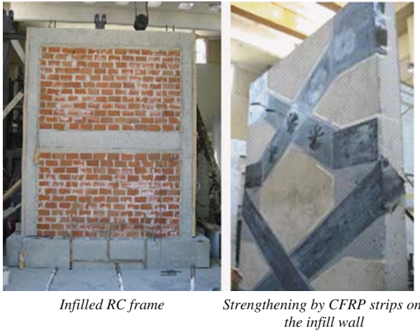
Fig. 19.27 Strengthening two story – one bay specimens (See also Plate 41 in Color Plate Section on page 477)
