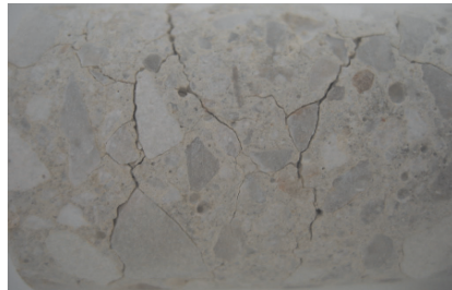
Fig. 4. Photograph of a small cylinder of concrete CEMII/59 subjected to cycles of immersion-drying at 60°C
