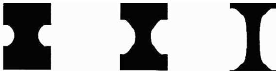
Fig. 4. Necking formation in specimens during tensile test
