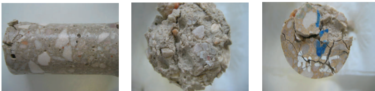
Fig. 3. Photographs of a small cylinder of concrete CEMII/59 subjected to total immersion at the end of test
