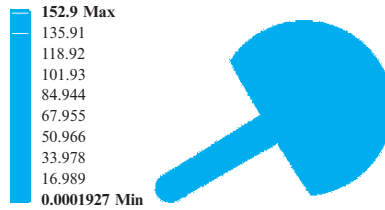
Fig. 7b. Von Mises stress in the trabecular bone using the hybrid composite-Co-Cr HR implant
