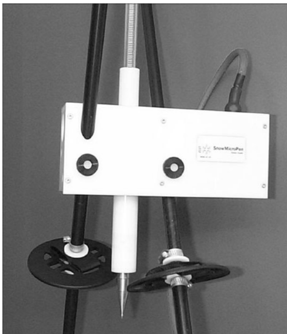
Snow Pit, Figure 3 SnowMicroPen (SMP) motor, sensor assembly. (Courtesy Schneebeli, M, SLF, Davos, Switzerland.)
