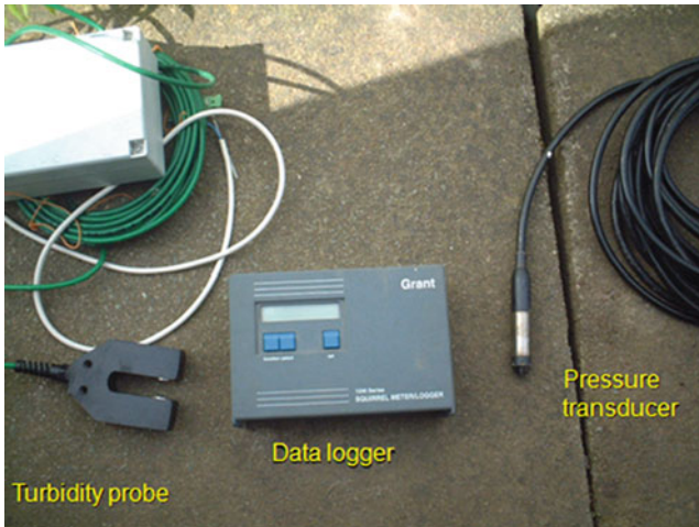
Suspended Sediment Dynamics, Figure 4 Partech turbidity sensor, data logger, and pressure transducer (photo: T. Stott).
