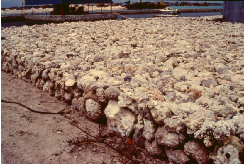
Mining/Quarrying of Coral Reefs, Figure 3 Weathering of coral rock prior to its use in construction in the Maldives.
