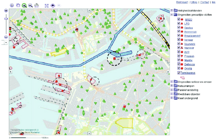
Fig. 13.5 Example of a Risk map. The symbols in red represent the hazardous establishments with the corresponding risk areas. The symbols in green indicate vulnerable public buildings, such as schools, hospitals, etc
