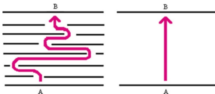
Fig. 5.38 Schematic representation of the gas path in a nanocomposite (path of the penetrant = d' ) and in a pure polymer (path of the penetrant = d )
