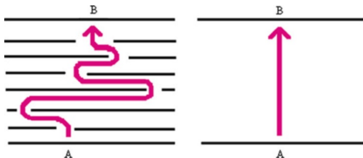
Fig. 5.38 Schematic representation of the gas path in a nanocomposite (path of the penetrant = d' ) and in a pure polymer (path of the penetrant = d )
