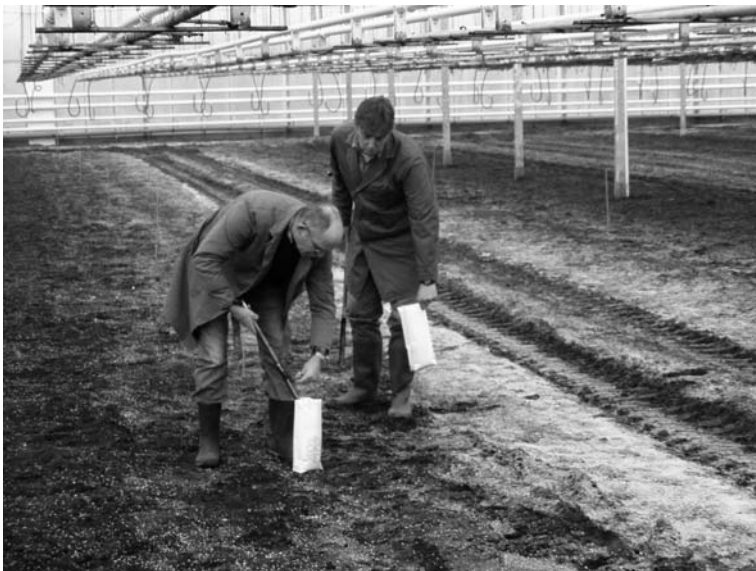
Picture 4.3 Soil sampling in a greenhouse. Generally, the sampling depth is 0.25 m
