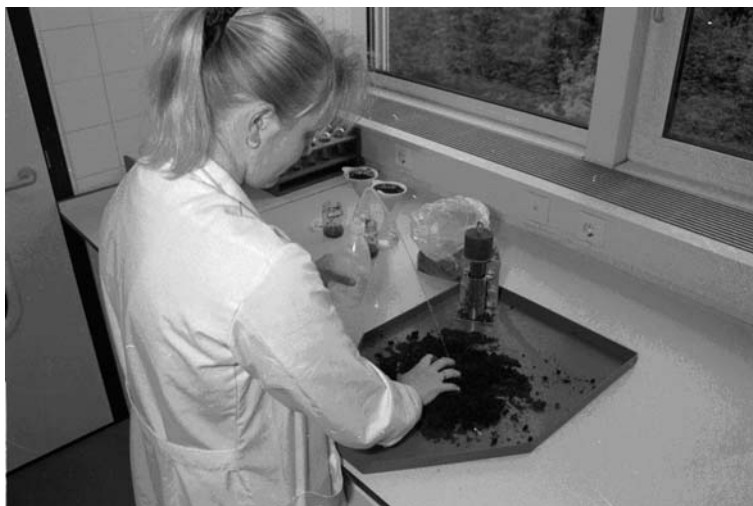
Picture 4.2 Preparation of the 1:1½ extract of peaty growing media. One volume of growing media is mixed with 1½ volume of water. The moisture contents of the growing media are adjusted to a pressure head of -3.2 kpa
