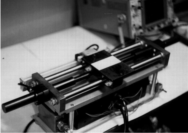
Fig. 6.17 General view of long travel magnetic rheology drive.
