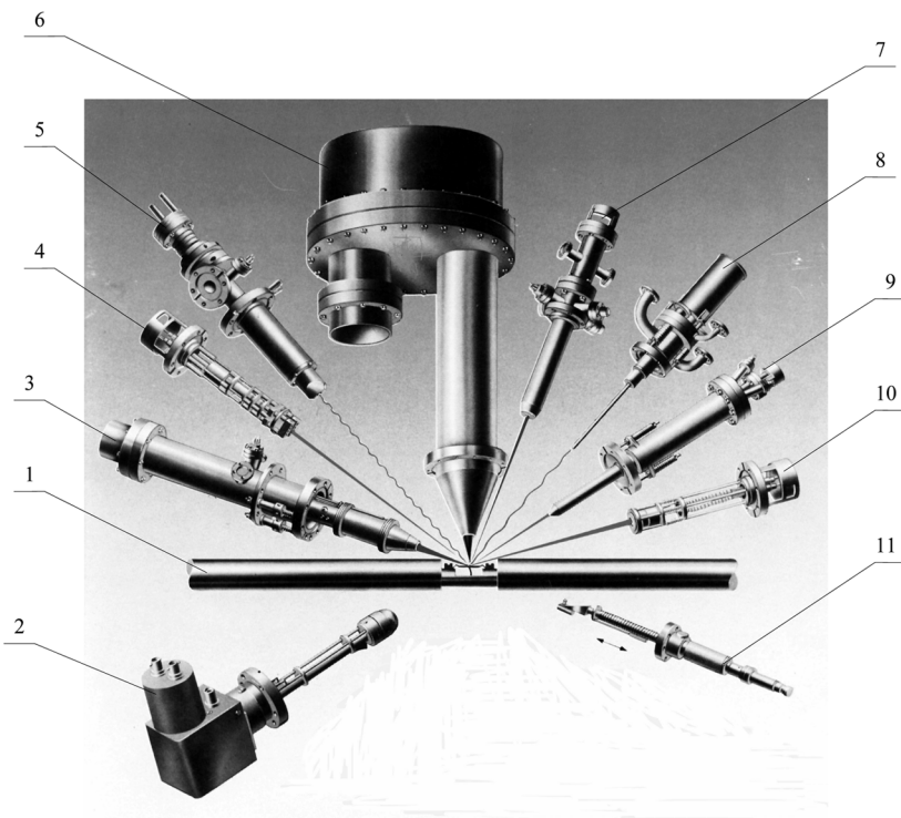
Fig. 1.12 The scheme of the research and technology instruments positioning [7] in vacuum about the searched wafer: 1 – searched wafer; 2 – detector of the secondary ions; 3 – secondary ions mass-spectrometer; 4 – electron gun for Auger analysis; 5 – X-ray source; 6 – energy analyzer; 7 – ion gun; 8 – ultraviolet source; 9 – micro focus electron gun; 10 – electron gun; 11 – Faraday cup.
