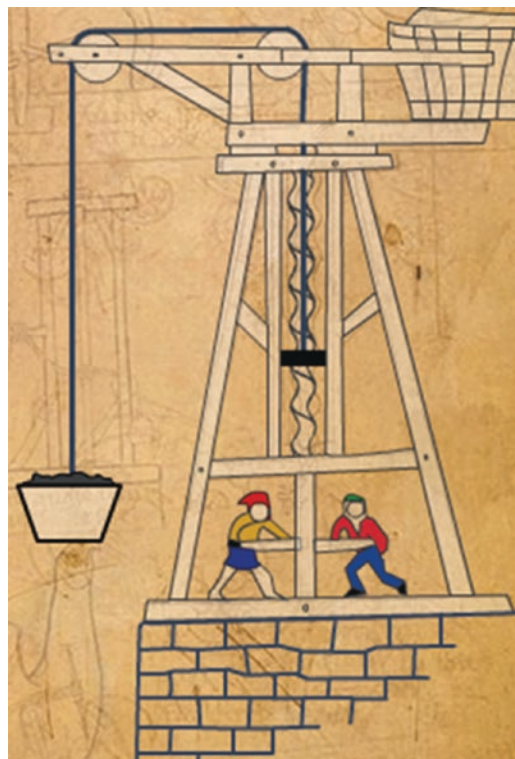
Fig. 4.27 Illustration of Villard de Honnecourt's elevator. Reconstruction by the BNF
