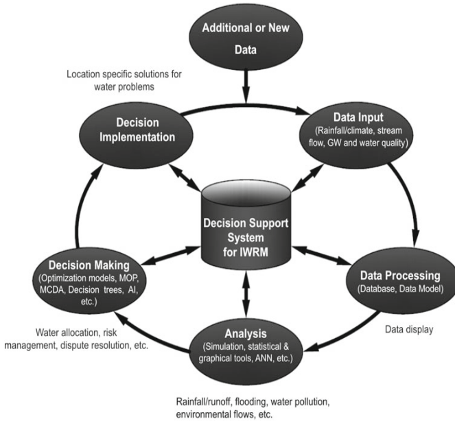
Fig. 4 General framework of a decision support system for water resources management (McKinney, 2004).
