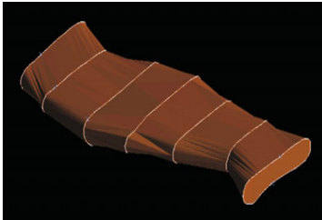
Fig. 16 Solid modeling and block modeling of an iron ore deposit using SURPAC.
