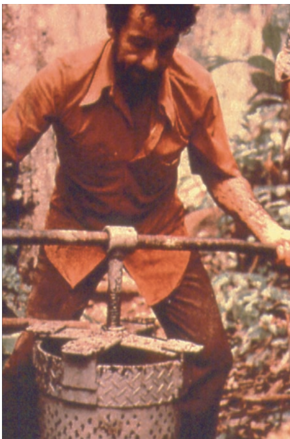
Fig. 20 A “cocinero” pressing the soaked leaves to separate out the kerosene containing the alkaloids (“La Prensa”) in a typical cocaine jungle laboratory
