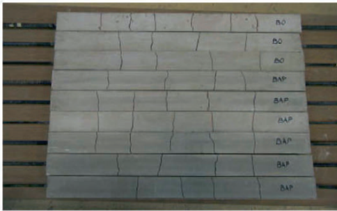
Figure 13. Experimental results of tension test on RC tie-beams producing variable values of crack spacing (from Daoud [2003], doctoral thesis INSA Lyon)
