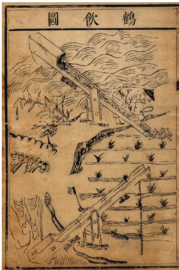
Fig. 3 Flume-beamed swape ( Xinzhì Zhuqì Tushuo , Lailutang edition)
