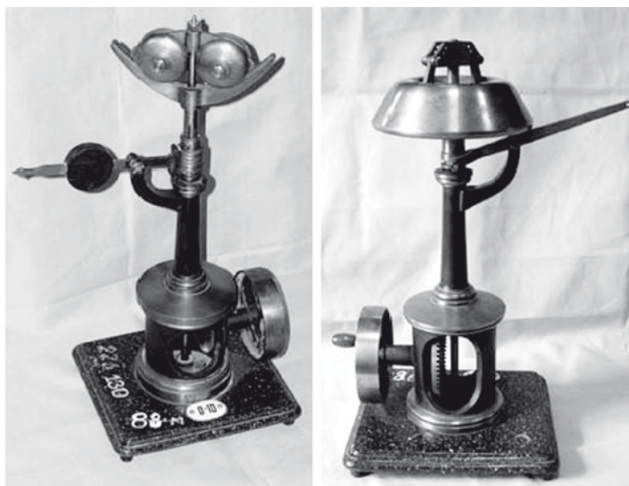
Fig. 9 The models of centrifugal governors, which were purchased by Orlov in Germany
