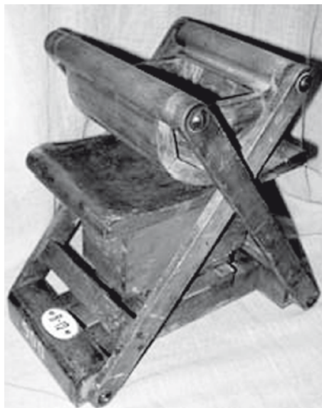
Fig. 7 Model of Chebyshev's "Excerpts from the Roulette theory" antiparallel link mechanism
