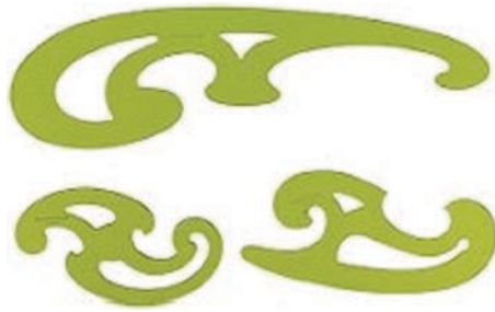
Fig. 10 A commercial set of Burmester templates (Courtesy of Faber-Castell)
