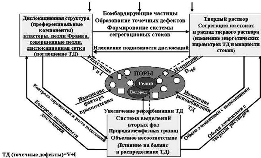
Fig. 7 Main relations in structure of irradiated stainless steels [2]
