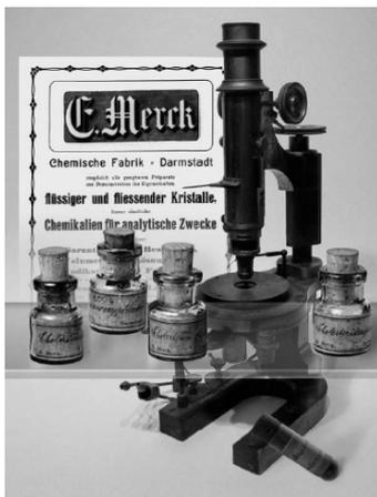
**Fig. 1.1** Lehmann's original hot-stage microscope and some Merck LC substances from 1904. Picture source: Merck KGaA, Corporate History
