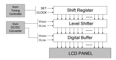
Fig. 6.36 Block diagram of the gate driver
