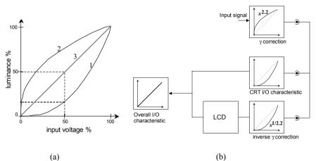
**Fig. 4.16 (a)** CRT luminance versus input voltage: (1) actual curve,  $x^{\gamma}$ , (2) gamma correction curve,  $x^{1/\gamma}$  and (3) ideal (linear) response, x. (b) TV broadcasting system. LCD is assumed linear but requires its own  $\gamma$  correction
