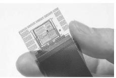
Fig. 5.4 CG Silicon CPU formed on a glass substrate (Semiconductor Energy Laboratory) [N2003]
