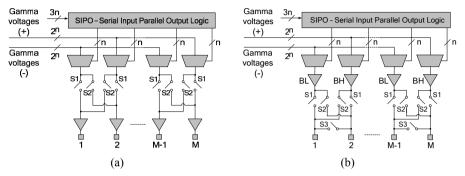
Fig. 6.23 Polarity inversion implementation with polarity reversal switches: (a) at the input and (b) at the output of the buffer amplifiers
