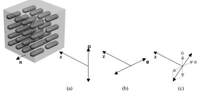
Fig. 1.23 Linearly polarized light entering an LC medium with  $\alpha = 90^{\circ}$ : (a) Pure ordinary wave. (b) Pure extraordinary wave. (c) Generic wave made up of ordinary and extraordinary components
