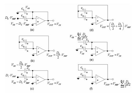
**Fig. 6.22** Conversion steps of the offset-compensated charge redistribution DAC. Output and capacitor voltages are indicated
