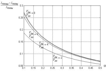
Fig. 7.15 Increment of current consumption (i.e., power consumption) in the case of area minimization with respect the case of minimum current consumption
