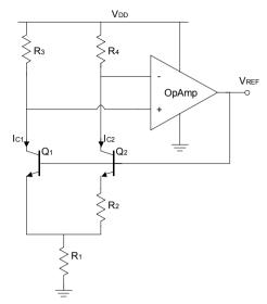
Fig. 4.4 Bandgap voltage reference with bipolar transistors
