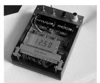
Fig. 2.7 TN LCD prototype presented by Helfrich and Schadt to the board of directors at Hoffmann-La Roche
