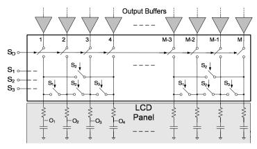
Fig. 6.34 Multiphase charge sharing circuit
