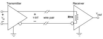
Fig. 6.10 Single transmission line of an LVDS system
