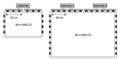
Fig. 6.7 82-in. AMLCD with two TCON PCBs
