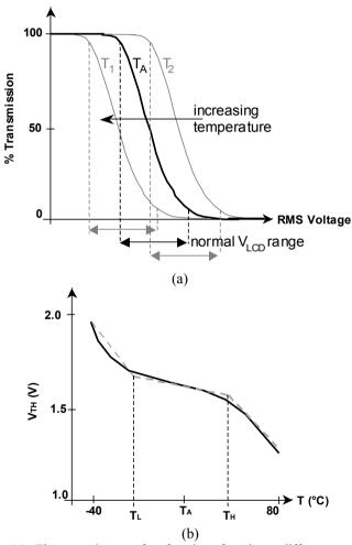
**Fig. 4.7** (a) Electro-optic transfer function for three different temperatures,  $T_1 > T_A > T_2$ , highlighting the associated  $V_{LCD}$  ranges. (b) Threshold voltage versus temperature (*solid line*), and a possible segmentation (*dashed line*)
