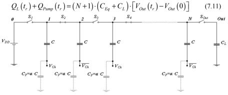
Fig. 7.7 N-stage CP with parasitic effects
