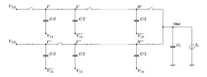
Fig. 7.22 Simplified schematic of a double CP
