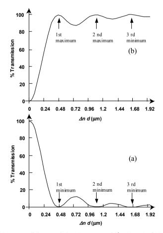
Fig. 2.10 Percentage light transmission, *T*, versus  $\Delta n d$  ( $\lambda = 555$  nm) of (a) normally white TN cell, (b) normally black TN cell. First, second, and third minima (maxima) are indicated
