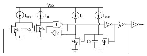
Fig. 4.13 Schematic of a relaxation oscillator [P2002]
