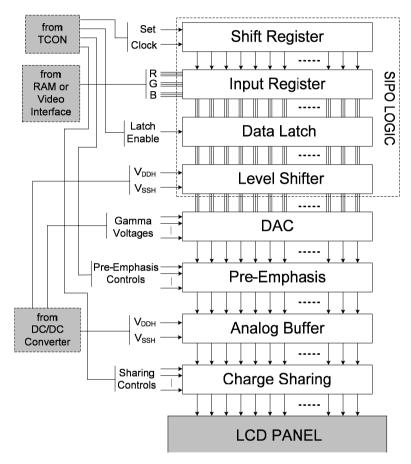
Fig. 6.15 Source Driver architecture of large size AMLCDs
