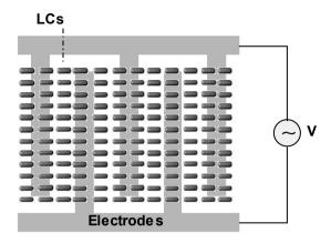
Fig. 2.23 In Plane switching electrodes scheme, top view. Typical electrode width is 4  $\mu$ m and electrode gap is 8  $\mu$ m
