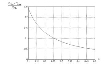
Fig. 7.9 Increase on total CP capacitance (proportional to silicon area) of minimum power consumption design with respect to the minimum area design
