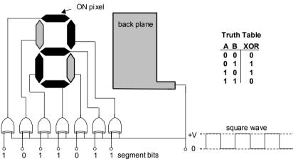
Fig. 3.3 Simple driving circuit for a seven-segment LCD
