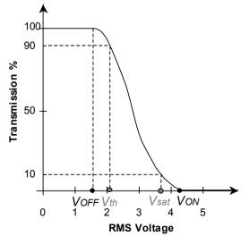
Fig. 3.11 Transmission as a function of the RMS applied voltage with superimposed  $V_{ON}$  and  $V_{OFF}$  values
