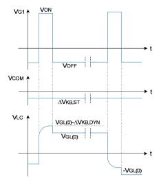
Fig. 5.21 Driving voltages in the case of 2-Level approach for a Cap-on-Common LCD panel structure
