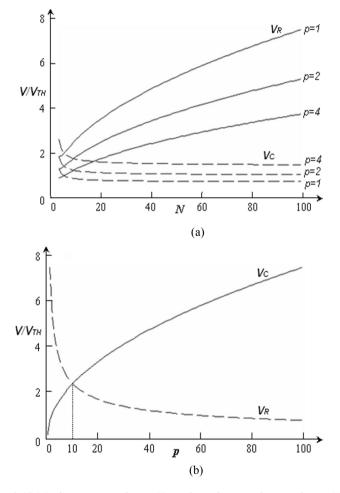
Fig. 3.17 Maximum row voltage,  $V_R$ , and maximum column voltage,  $V_C$ , normalized to  $V_{TH}$ . (a) plotted versus N for p=1, 2 and 4, (b) plotted versus p for N=100
