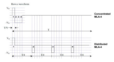
**Fig. 3.15** Row-a waveform of Fig. 3.14 for a Concentrated MLA-4 approach (upper trace) and Distributed MLA-4 approach (lower trace)
