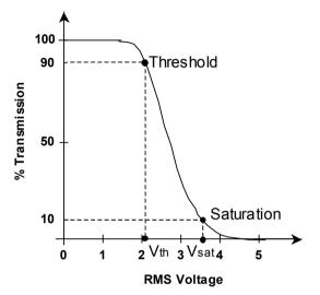
**Fig. 2.11** Electro-optic transfer function (EOTF) for a typical normally white TN cell showing Transmission as a function of the RMS applied voltage (at 1 kHz)
