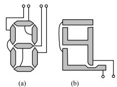
Fig. 3.5 Segment scheme for 1/2 duty-cycle drive: (a) upper and (b) lower electrodes
