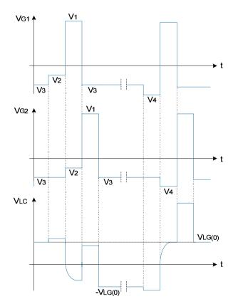
Fig. 5.28 Driving and pixel voltages in the case of 4-level driving scheme. Frame Inversion is considered
