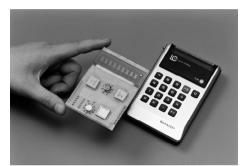
Fig. 2.6 The first liquid-crystal pocket calculator, which used DSM. Courtesy of Sharp Corporation
