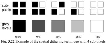
Fig. 3.22 Example of the spatial dithering technique with 4 sub-p
