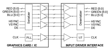
Fig. 6.11 Example of 18-bit LVDS interface
