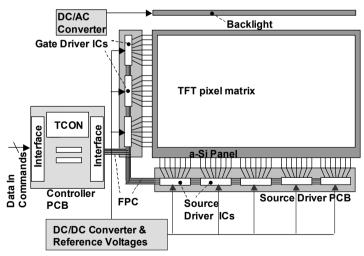
Fig. 6.5 Typical multichip driver architecture for large-area AMLCDs
