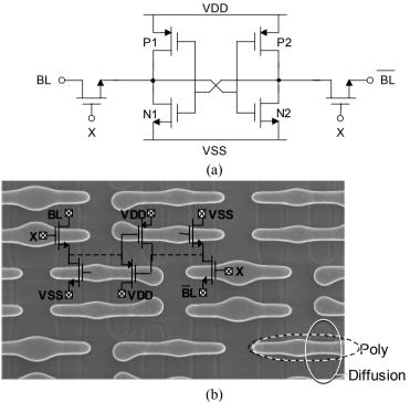
Fig. 4.22 (a) SRAM cell schematic, (b) micrograph of a SRAM bank in HVG8 technology
