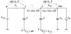
Fig. 7.12 A two-stage CP with a current load
