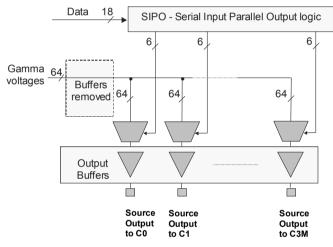
Fig. 6.19 Distributed buffer architecture
