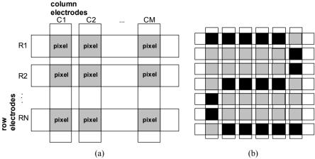
Fig. 3.6 Passive matrix LCD: (a) schematic representation of the pixels made up of orthogonal rows and columns of electrodes, (b) example of a displayed numeral
