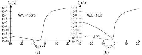
Fig. 5.5 Drain current versus gate-source voltage for an n-channel TFT: (a) a-Si TFT with W/L=100  $\mu$ m/5  $\mu$ m and (b) poly-Si with W/L=10  $\mu$ m/5  $\mu$ m. Voltage  $V_{DS}$  is 5 V in both cases. The *dashed curve* in (b) represents the OFF current obtained with lightly doped drain (LDD) technology
