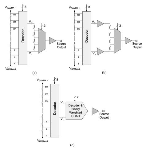
**Fig. 6.20** Two-stage DACs: (a) 8-bit R-DAC followed by a 2-bit R-DAC; (b) 8-bit R-DAC followed by a 2-bit R-DAC with intermediate buffers; (c) 8-bit R-DAC followed by a 2-bit binary weighted capacitor DAC
