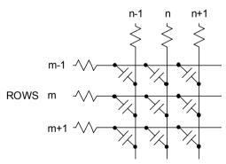
Fig. 3.20 Electrical model of a PM-LCD panel
