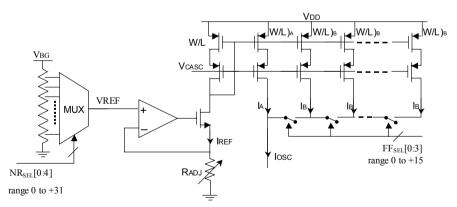
Fig. 4.14 Scheme for the generation of *I*<sub>OSC</sub>
