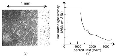
**Fig. 2.1** Williams experiment: (a) Williams domains. In the *left dark area*, a 1-kHz AC field of 2500 V/cm directed perpendicular to the plane is applied through transparent electrodes. Parallel regions (domains) are apparent. The *bright area at the right* is without the transparent conductive coating, therefore there is no field applied. Sample thickness is about 50  $\mu$ m and temperature is 125°C. (b) Qualitative behaviour of transmitted light versus the electric field
