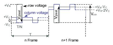
Fig. 3.10 Row and column voltages used to switch ON a pixel in the case of IA&P technique
