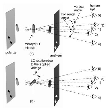
Fig. 2.14 Illustration of horizontal and vertical viewing angles: (a) The mid-layer LC molecule is vertical with respect to the observer at any position and therefore the same birefringence is experienced (same gray level). (b) Rotation of the mid-layer LC molecule causes a considerable difference in birefringence but only for vertical viewing angles
