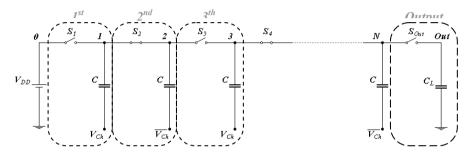
Fig. 7.4 *N*-stage charge pump
