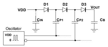
Fig. 4.10 Simplified scheme of a ×3 charge pump
