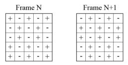
Fig. 5.17 Vertical 2-Dot Inversion driving method
