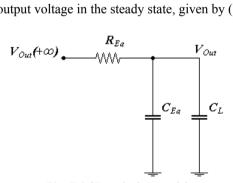
Fig. 7.6 CP equivalent model
