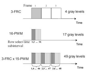
Fig. 3.26 Example of 3-FRC and 16-PWM mixed technique to display 49 gray levels
