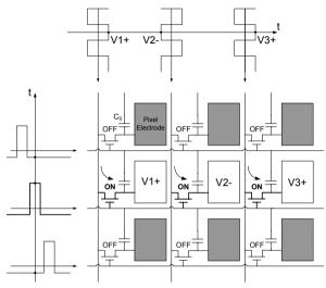
Fig. 5.10 Addressing example of an Active Matrix LCD
