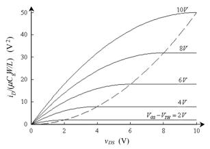
Fig. 5.2 Output characteristics (drain current versus drain-source voltage) of a generic TFT for  $V_{GS} - V_{TH} = 2, 4, 6, 8, 10 \text{ V}$
