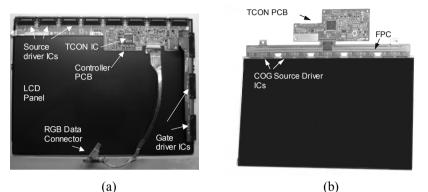
**Fig. 6.9** Photographs of AMLCD panels for notebook computers with driving circuitry: (**a**) 14-in. conventional style; (**b**) 12.1-in. with integrated a-Si Gate Drivers and COG PAD ring of Source Drivers by Samsung [BMK2005]
