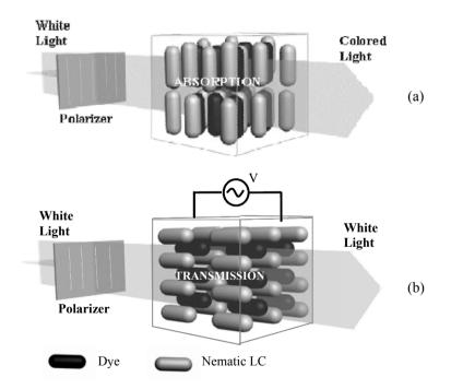
**Fig. 2.2** The guest-host effect: (a) With no applied voltage, the direction of polarization of linearly-polarized light is parallel to the molecules long axis (i.e., it is vertical), some light frequencies are hence absorbed by the dye and the cell appears colored. (b) With an applied voltage, the direction of polarization of linearly-polarized light is parallel to the molecules long axis. Light is completely transmitted and the cell appears transparent
