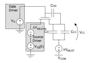
Fig. 5.18 Kickback compensation through the Source Driver (dynamic part) and  $V_{COM}$  (static part). The static part can be also compensated via the subsequent gate line, for cap-on-gate architectures
