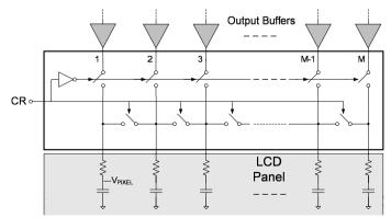
Fig. 6.30 Simple charge sharing circuit
