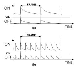
Fig. 3.16 Time distribution of pixel voltages in: (a) the A&P technique, and (b) MLA-4 technique
