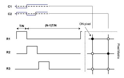
Fig. 3.7 Simple row and column waveforms for a passive matrix LCD
