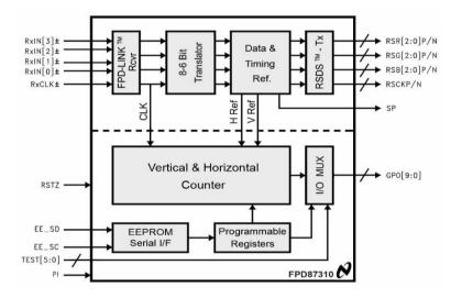
Fig. 6.6 Example of fully integrated TCON IC from National Semiconductor Corp [LL2000]
