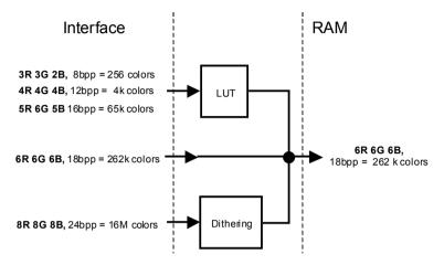
Fig. 4.2 Example of LUT/Dithering operation required in the case of a 18-bit video RAM
