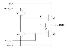
Fig. 6.40 Schematic of the a-Si shift register cell with bootstrap
