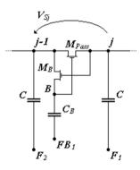
Fig. 7.21 Generic stage (plus a capacitor) of a bootstrap CP
