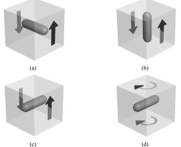
**Fig. 1.16** Graphical examples of translational and rotational viscosity coefficients in LCs: (a)  $\eta_1$ , (b)  $\eta_2$ , (c)  $\eta_3$  and (d)  $\gamma$
