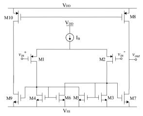
Fig. 6.14 Schematic diagram of LVDS receiver based on a Schmitt trigger (termination resistor  $R_{TR}$  is not shown) [USS1996]
