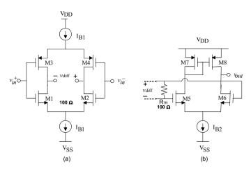
Fig. 6.12 Simplified LVDS transmitter (a) and receiver (b)
