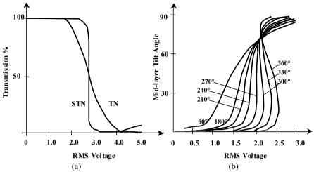
**Fig. 2.19** (a) Transmission as a function of the RMS applied voltage (at 1 kHz) for a typical normal white TN (twist angle=  $90^{\circ}$ ) cell and STN (twist angle =  $270^{\circ}$ ) cell. (b) Tilt angle of the LC mid-layer molecules as a function of the RMS applied voltage for different twist angles
