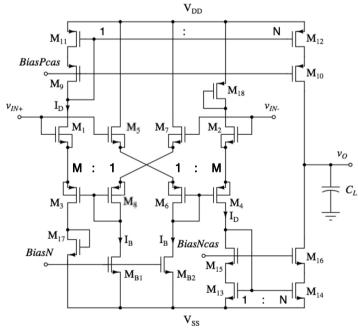
Fig. 6.29 Schematic of the transconductance amplifier in [DPS2007]
