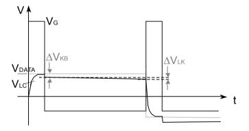
Fig. 5.12 Qualitative behavior of the pixel voltage due to kickback and leakage
