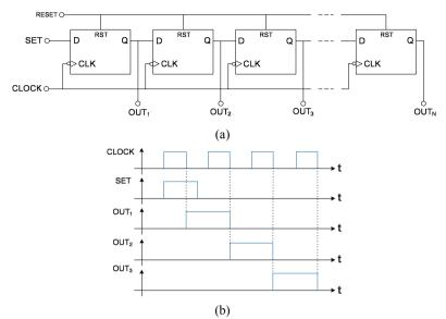
Fig. 6.37 Flip flop shift register: (a) block diagram and (b) waveforms
