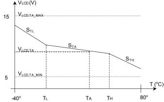
Fig. 4.9 Example of a segmented temperature programmable  $V_{LCD}$  voltage. The temperature range is split into three segments. Parameters  $V_{LCD,TA}$ ,  $S_{TL}$ ,  $S_{TA}$  and  $S_{TH}$  are the only stored into the OTP
