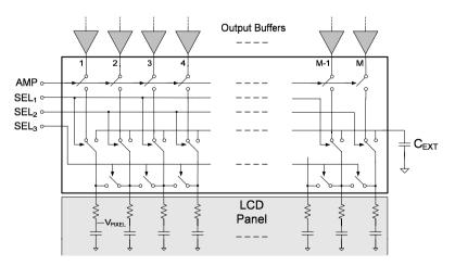
Fig. 6.32 Triple charge sharing circuit
