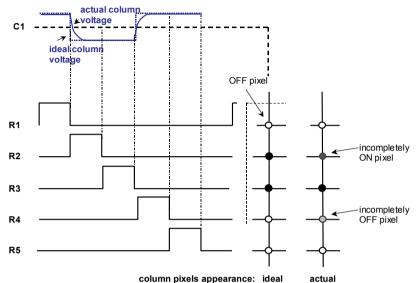
**Fig. 3.21** Effect of the RC delay onto the pixel driving voltages. The ideal pixel appearance and actual one are compared at the right. Pixels driven in presence of a column transition can receive more (row 4) ore less (row 2) energy
