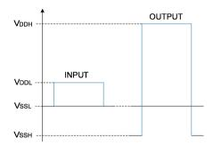
Fig. 6.42 Input and output waveforms of Level Shifter
