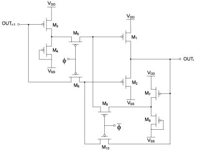
Fig. 6.39 Schematic of the LTPS shifter register cell
