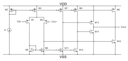
Fig. 6.27 Class-AB two-stage amplifier
