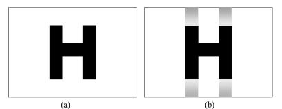
Fig. 3.19 Example of effects of crosstalk: (a) ideal picture, (b) picture with vertical crosstalk
