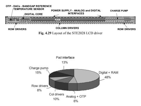
Fig. 4.30 Block partitioning of the STE2028 LCD driver
