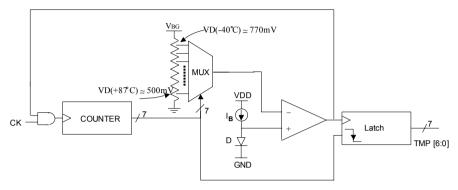
Fig. 4.8 Block scheme of the Temperature Sensor
