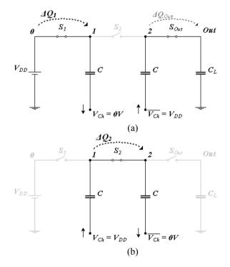
Fig. 7.5 *N*-stage CP: (a) first half period; (b) second half period
