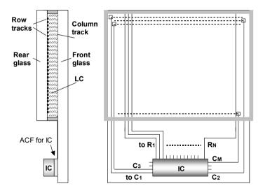
Fig. 4.27 LC panel with COG driver IC
