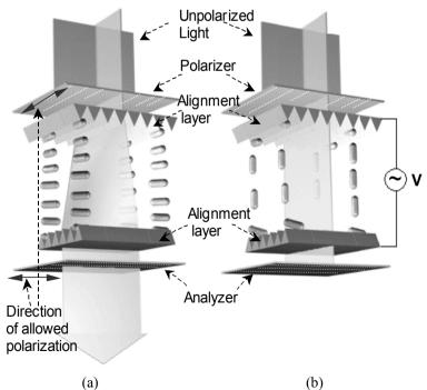
**Fig. 2.9** The Twisted Nematic effect in a normal white cell: (a) The direction of polarization of the light entering the liquid-crystal region rotates by  $90^{\circ}$  along the helix arrangement of the LC molecules and the screen appears *white*. (b) Light is blocked by the analyzer and the cell appears *black*
