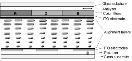
Fig. 2.20 The use of RGB filters to realize a color TN LCD
