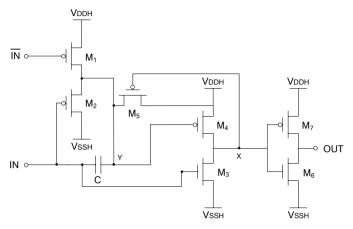
Fig. 6.45 Schematic of an LTPS level shifter [LJ2006]
