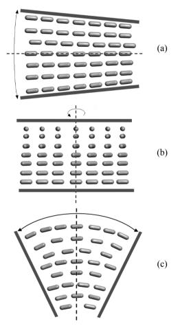
Fig. 1.13 Molecular alignments of nematic liquid crystals under external mechanical stress: (a) splay, (b) twist, (c) bend [F1958]
