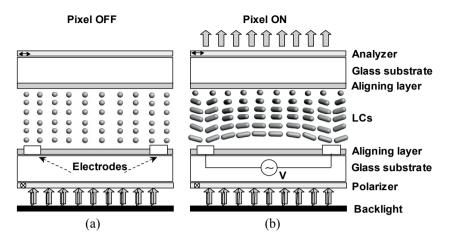
Fig. 2.22 In Plane Switching cell. (a) OFF state, (b) ON state. Cross-oriented polarizing filters are used. Electrodes are placed only in the back plane and align in the same plane the LC molecules
