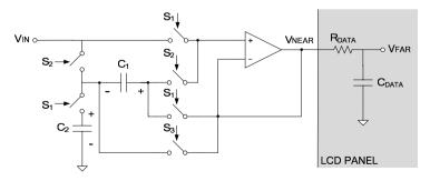
Fig. 6.24 Circuit diagram for the pre-emphasis driving method
