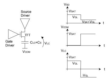
Fig. 5.22 Source Driver and V<sub>COM</sub> waveforms for V<sub>COM</sub>-switching driving scheme
