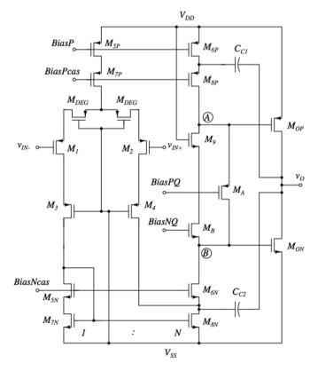
Fig. 6.28 Schematic of the transconductance amplifier in [B2005]
