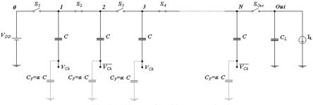
Fig. 7.11 N-stage CP with a current load
