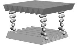
Fig. 2.8 Representation of the  $90^{\circ}$  helical rotation of LC molecules in Twisted Nematic cells
