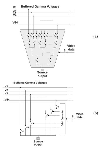
Fig. 6.18 Implementation of the multiplexers with: (a) binary tree switches, (b) with decoder
