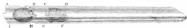
Figure 9.1 Leeuwenhoek's (1695) test set-up to examine the acaricidal effects of nutmeg on mites, consisting of a glass tube ca. 13 inches long, closed at one end (E), containing about 150 000 mites and some pieces of nutmeg (A–B, C–D). (From Hoole, 1798; Plate 10, Figure 1, p. 289 et seq. )
