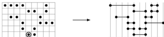
Figure 2.1. Left: a directed animal on the King's lattice (represented, for clarity, as a polyomino on the dual lattice) with its source circled. Right: the pyramid of segments obtained by replacing each maximal sequence of \ell consecutive sites by a segment of length \ell .
