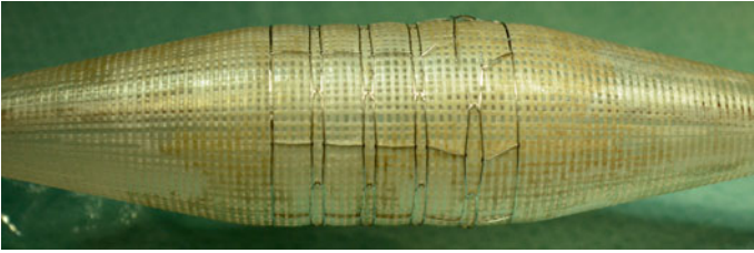
Fig. 21.3 A Cook Formula stent dilated on a 18 mm ultrahigh-pressure balloon. The stent struts begin to rupture and, thus, give way to unrestricted further dilation
