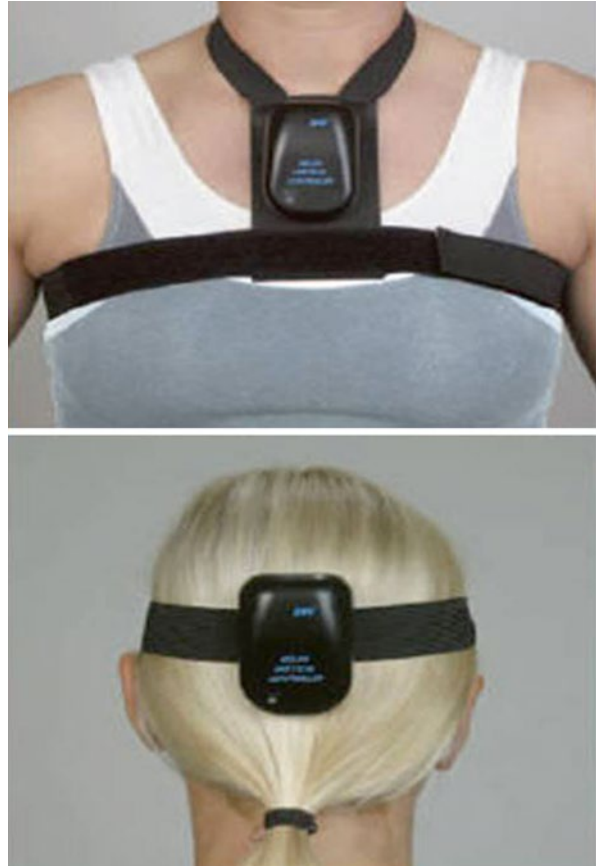
Fig. 19.6 An accelerometer is fixed on the head and the other on the trunk in order to record sagittal and lateral displacements of the two body segments
