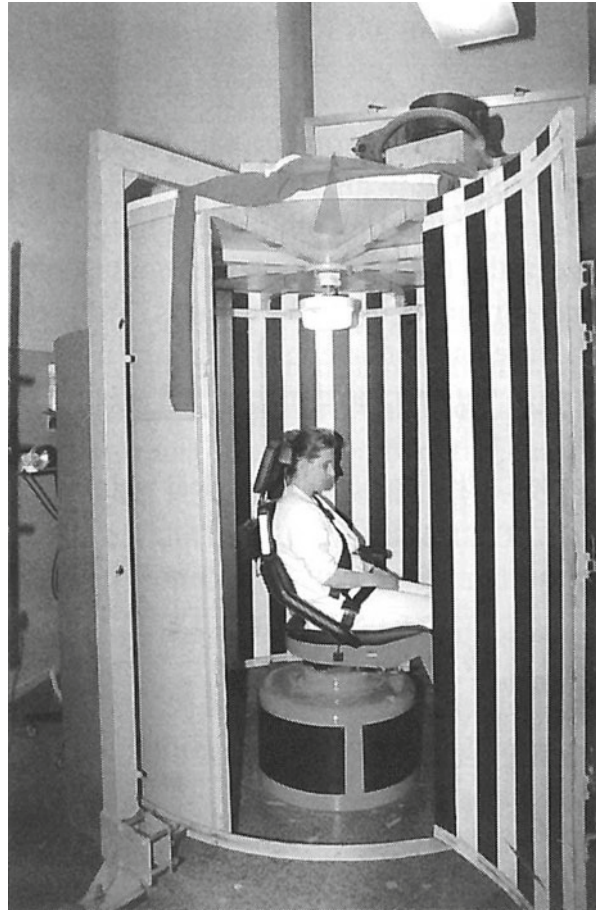
Fig. 23.1 Rotatory cylindrical chamber. The Tonnie's rotatory chair system Pro in the middle
