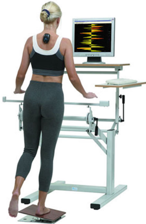
Fig. 26.1 Delos® equipment. Subject stands on the board with one or 2 ft and tries to maintain equilibrium. Body and board sway are contemporary recorded and presented as visual feedback in order to improve visual control of dynamic posture stabilisation
