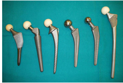
Fig. 4.5 Contemporary and historical femoral components documenting the wide variety of designs with various coatings reflecting different fixation methods
