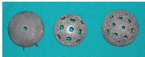
Fig. 4.6 View of the backside of new acetabular components with porous metal coatings
