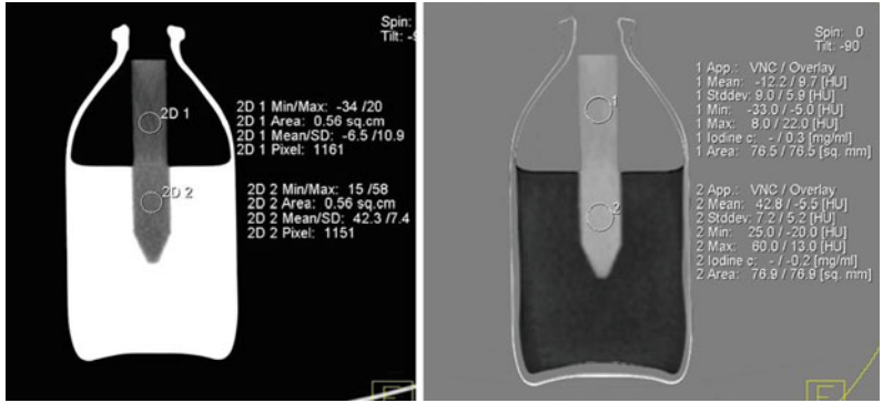
Fig. 3.17 Standard 120-kVp ( on the left ) and corresponding dual-energy color-coded iodine overlay ( on the right ) images of a phantom containing a vial of water immersed in an iodine solution (20 mg/mL). The lower ROI on the standard 120-kVp image clearly demonstrates
