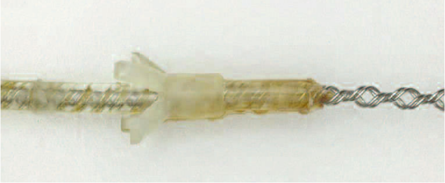
Fig. 23.2 An implanted tined lead broken during the removal procedure
