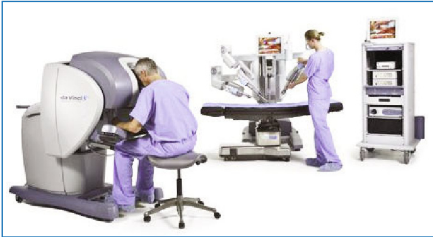
Fig. 15.1 The da Vinci TM robotic system (courtesy of Surgical Intuitive, Inc., Sunnyvale, CA, USA)
