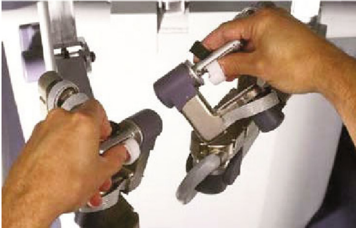
Fig. 15.3 The da Vinci dual-console surgical system (Master Handles) (courtesy of Surgical Intuitive, Inc., Sunnyvale, CA, USA)
