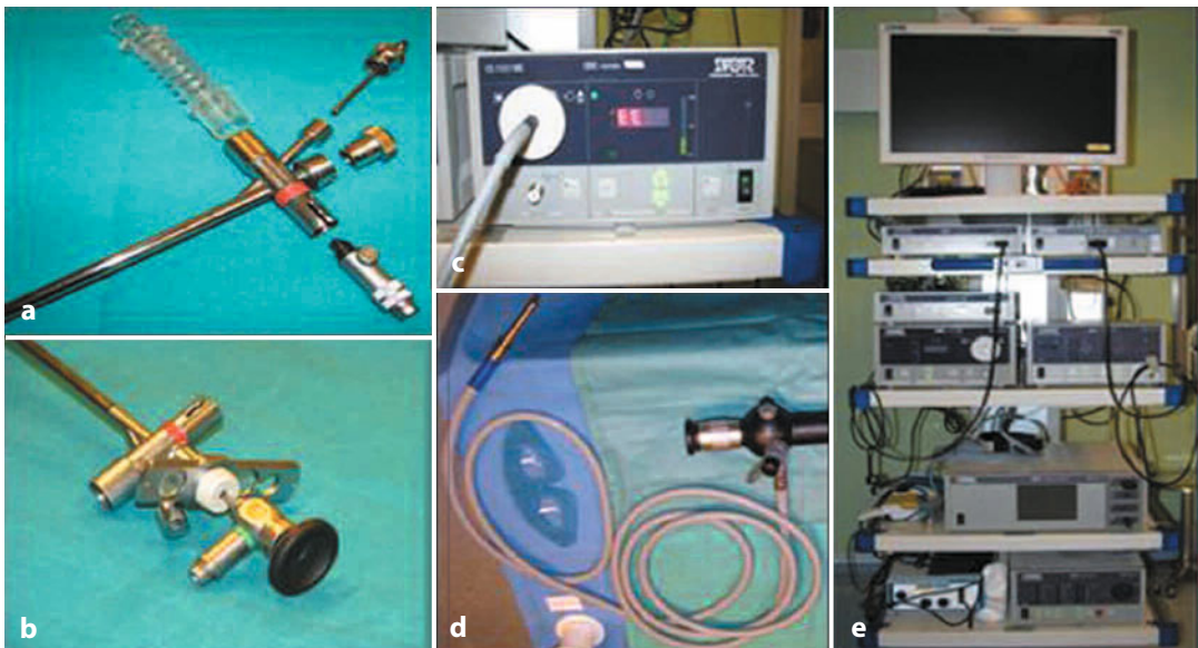
Fig. 15.3 Endoscopes and endoscopic system used for image acquisition. a,b Rigid endoscope. c Light source. d Flexible endoscope. e System for image acquisition
