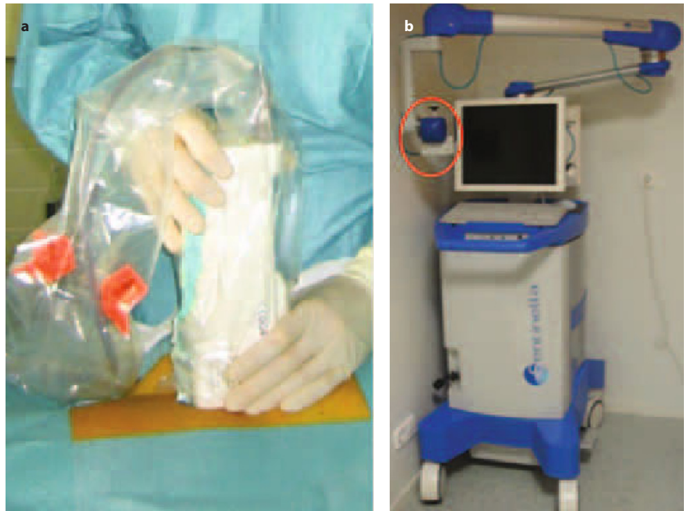
Fig. 7.10 Examples of portable gamma cameras. a light-weight portable gamma camera (less than 1 kg), without support system. b latest-generation portable gamma camera with improved ergonomometry and adequate and stable support system for intraoperative use; this unit incorporates a laser pointer to center the image and adjust the scanning procedure
