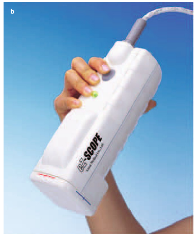
Fig. 3.5 a Latest-generation portable gamma camera with improved ergonomic details and adequate support system for intraoperative use. b Portable gamma camera weighing less than 1 kg but without a support system
