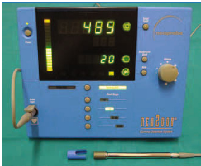
Fig. 3.4 Gamma probe Neo2000 from Neoprobe (Devicor Medical Products, Inc., Cincinnati, OH). The gamma probe (in the foreground) is shown with a removable collimator. Display of the control unit shows the count rate over 20-sec intervals, represented both with a numerical readout (at the center in the top of the monitor) and with an analog-like signal (vertical scale at the left of the monitor)
