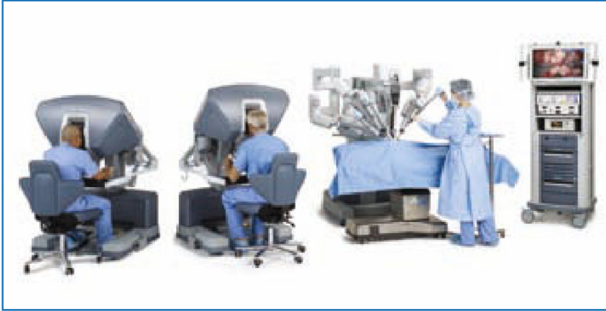
Fig. 4.1 da Vinci Surgical System Si HD (reproduced with permission from Intuitive Surgical, Inc.)
