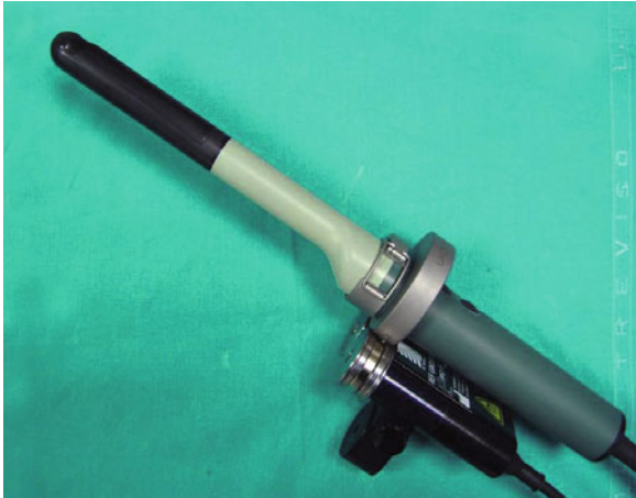
Fig. 6.11 The 180° rotational mover for 3D motorized acquisition is connected to the transducer type 8848 (B-K Medical) by using a magnetic disk
