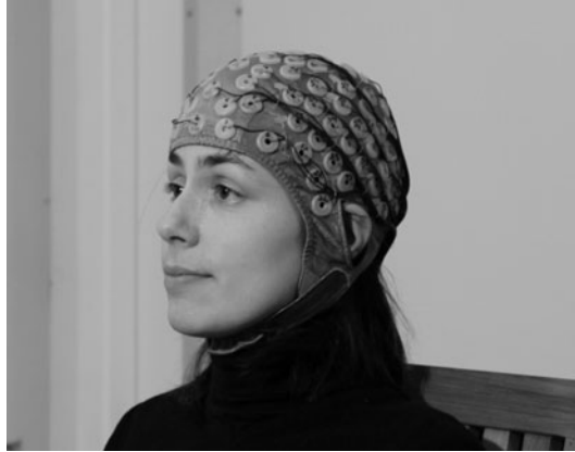
Fig. 9.14. The distribution of the sensors for EEG
