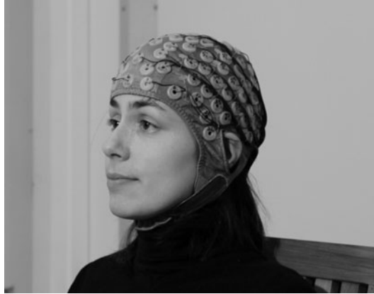
Fig. 9.14. The distribution of the sensors for EEG
