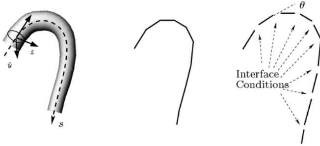
Fig. 10.5. Splitting of a curved domain into a sequence of rectilinear segments
