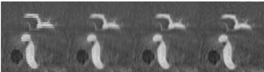
Fig. 4.6. From left to right, CRA image with anisotropic resolution (the number of points along the horizontal direction is four times greater than along the vertical direction), resampled with nearest neighbour, linear, cubic and sinc interpolation
