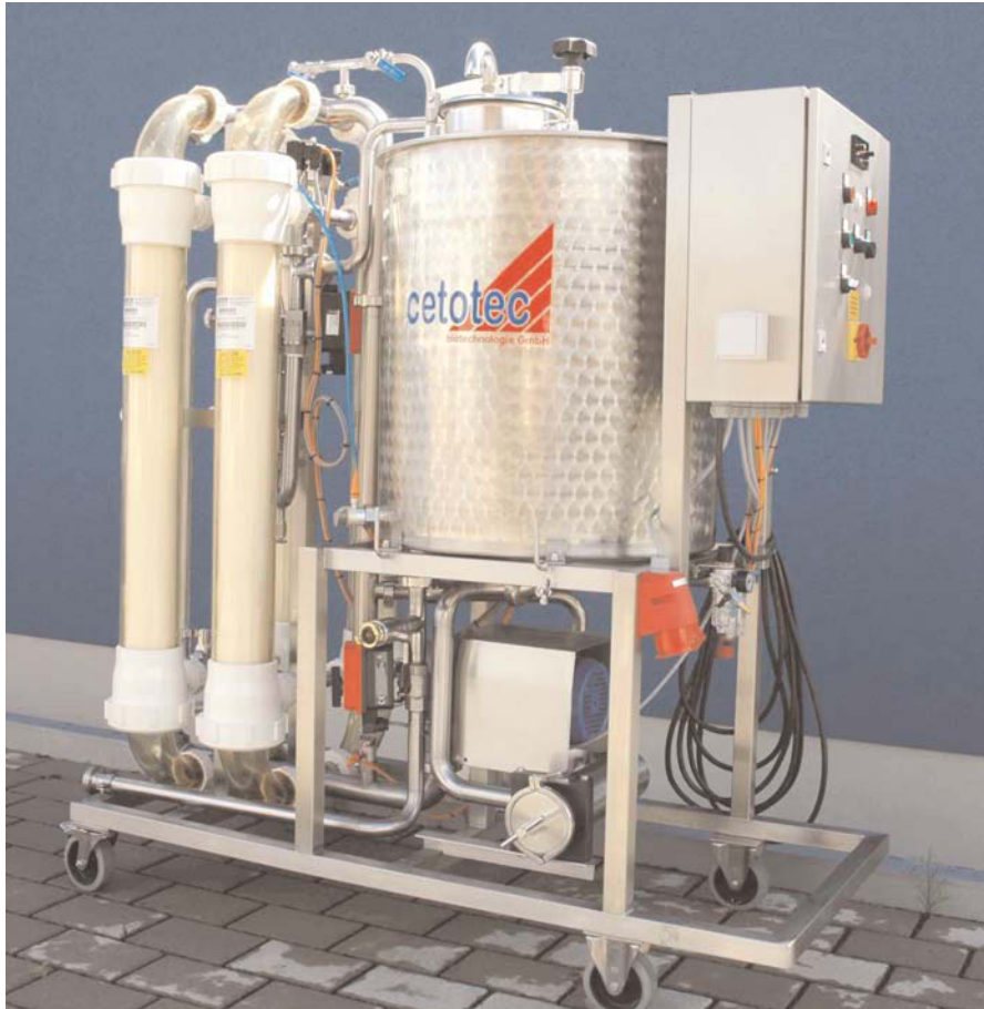
Figure 9.4 Model of a cross-flow filtration plant used for continuous microfiltration of vinegar
