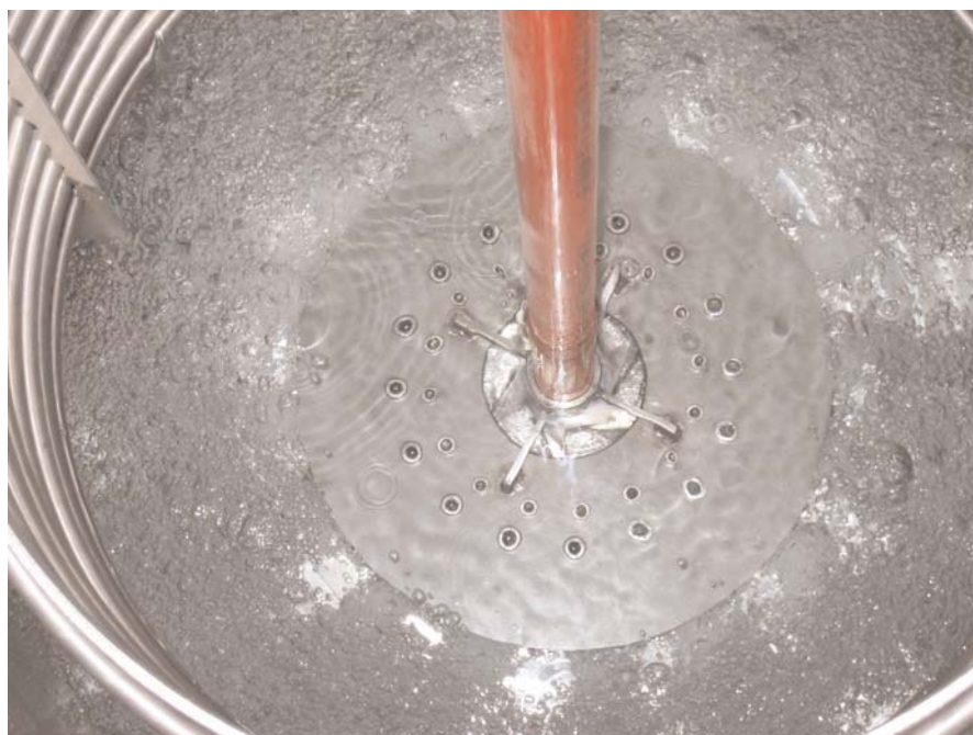
Figure 9.2 Highly efficient aeration system in a fermenter for wine vinegar production
