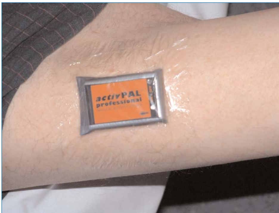
Fig.2. The activPAL™ professional physical activity logger attached to the front of the thigh
