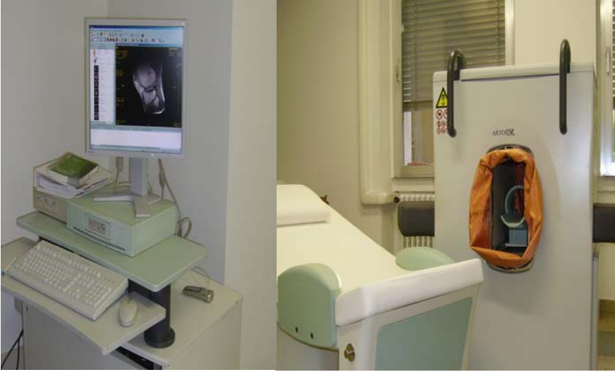
Fig. 1. MRI Artoscan (Esaote SPA Genova, Italy) Imager dedicated to the investigation of articular diseases. The system in the picture is placed in the NMR laboratory of the Department of Physics "A. Volta", University of Pavia, Italy.
