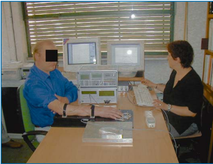
Fig. 7. A hand transplanted patient during kinetics assessment. Experimental setup and hand positioning on the instrumented keyboard
