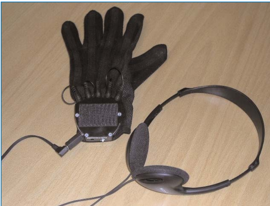
Fig. 1. The Sensor Glove equipped with stereo processor and ear phones. Miniature microphones are incorporated in the glove at fingertip levels
