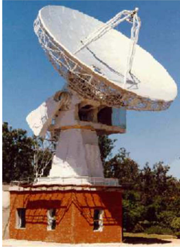
Fig. 5.31 A picture of the 10.4 m diameter millimetre wave dish located at the RRI campus. The 10.4 m dish was installed in RRI campus and has been in operation since 1988. At the highest operating frequencies, a closed cycle 4K helium cryogenic system has been used.
