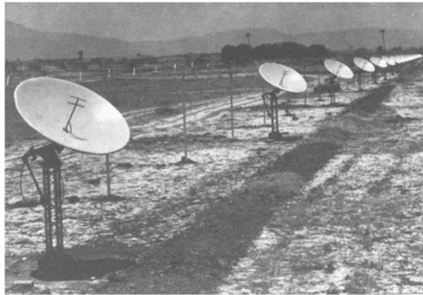
Fig. 5.1 Twenty-four dishes of the EW array of the Kalyan Radio Telescope at 610 MHz (Swarup et al. 1966)
