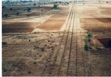
Fig. 5.22 An aerial view is shown of a section of the east-west arm of the Gauribidanur radio telescope operating at 34.5 MHz
