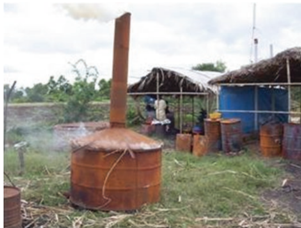
Fig. 6.1 An “oven and retort”-type kiln for charring agricultural waste
