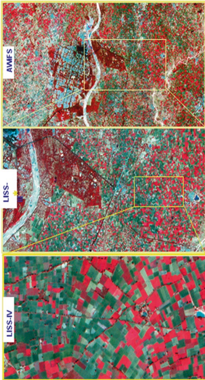
Fig. 22.3 The concept of imaging at different spatial resolutions suitable for resource mapping at variable scales as seen in FCC of AWiFS, LISS III, and LISS IV sensors over an area. The rectangle in the image highlights the reduction in area coverage as the spatial resolution increases
