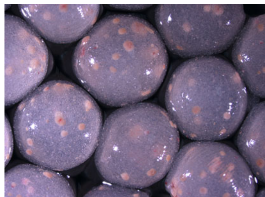
Fig. 14.2 Immobilization of microbial inoculants in calcium alginate beads by ionic gelation technique (beads 2–3 mm in diameter)
