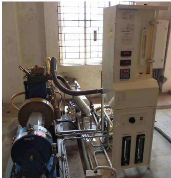
Fig. 2 Computerized engine coupled with eddy current dynamometer
