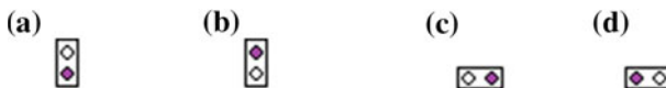
Fig. 1 2-dimensional 2-dot 1-electron QCA cells. a Vertically oriented cell with polarity '0'. b Vertically oriented cell with polarity '1'. c Horizontally oriented cell with polarity '0'. d Horizontally oriented cell with polarity '1'
