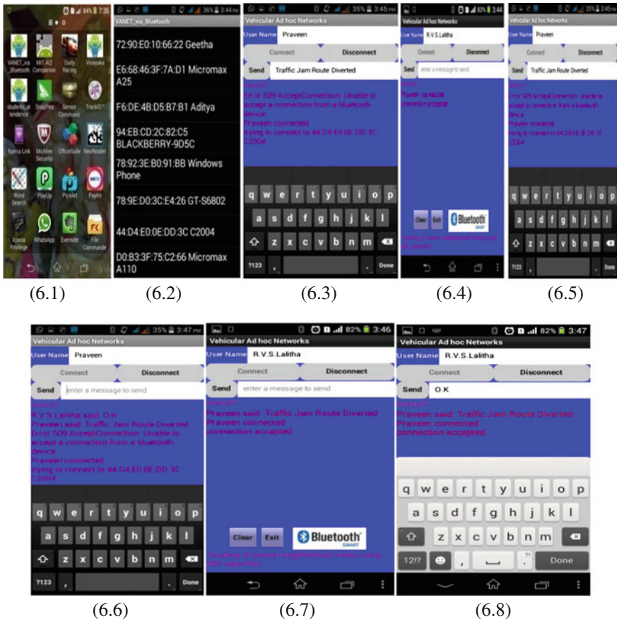
Fig. 6 Collection neighborhood information using bluetooth. a Displaying VANET_via_Bluetooth app in android mobile. b List of VANET nodes near by. c and d Pairing of two VANET nodes. e and f Accepting to communicate by two VANET nodes. g Transmission of message by VANET node. h Reception of message by VANET node
