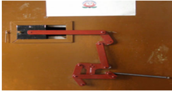
Fig. 3 Fabricated half scale model of switchgear mechanism used for opening operation
