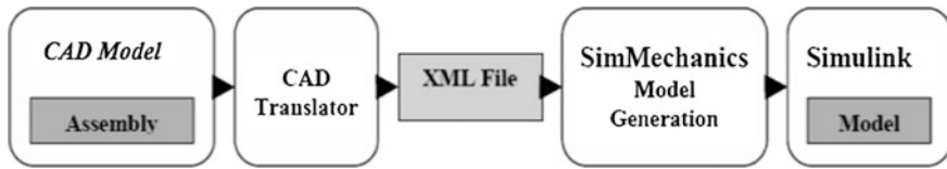
Fig. 3 Translating CAD model to SimMechanics
