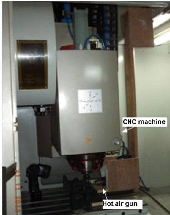
Fig. 2 Heating arrangement on CNC vertical milling machine using hot air gun
