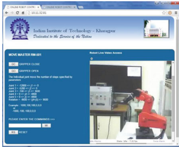
Fig. 9 Online robot control panel for Movemaster at client side with vision feedback system
