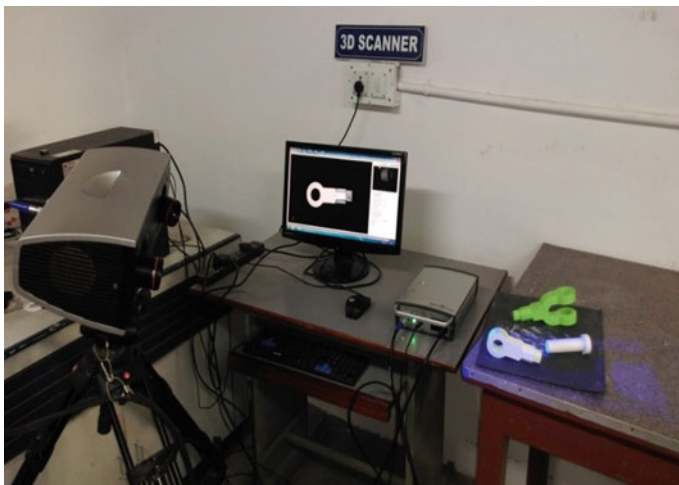
Fig. 2 Steinbichler COMET L3D-blue light scanner
