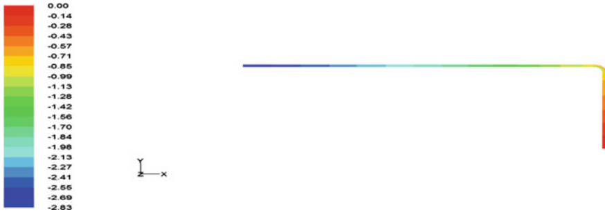
Fig. 3 Variation of Pressure drop at C_{vf} = 3.9\% and V_f = 1.8\text{ m/s}
