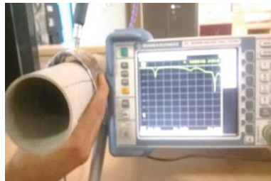
Fig. 11 Antenna under bending on 5 cm dia PVC pipe
