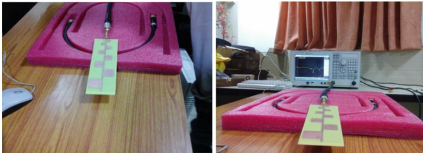
Fig. 7 Fabricated structure and experimental setup of frequency independent antenna
