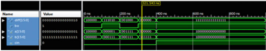
Fig. 13 Output response of 16-bit reversible subtractor
