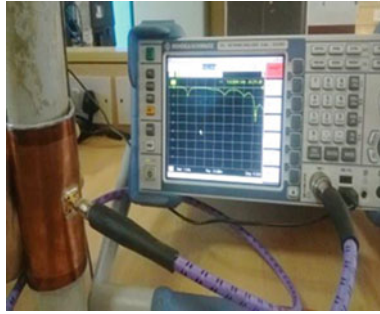
Fig. 9 Flexible software antenna placed on PVC pipe
