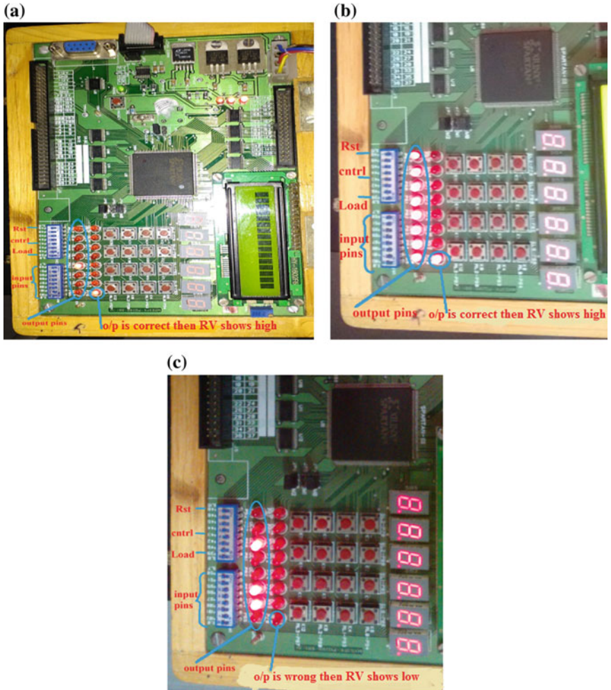
Fig. 9 a Normal mode on FPGA. b. Test mode on Spartan3 FPGA. c Fault condition in normal mode
